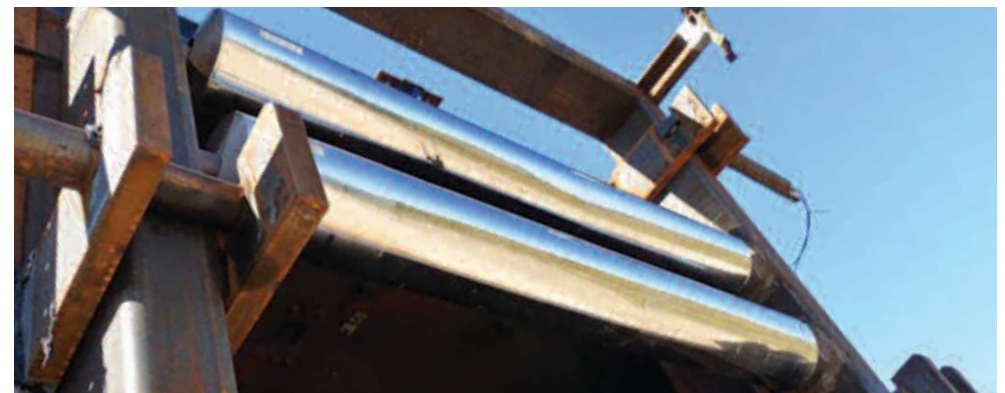
Pipe system after second explosion test.
