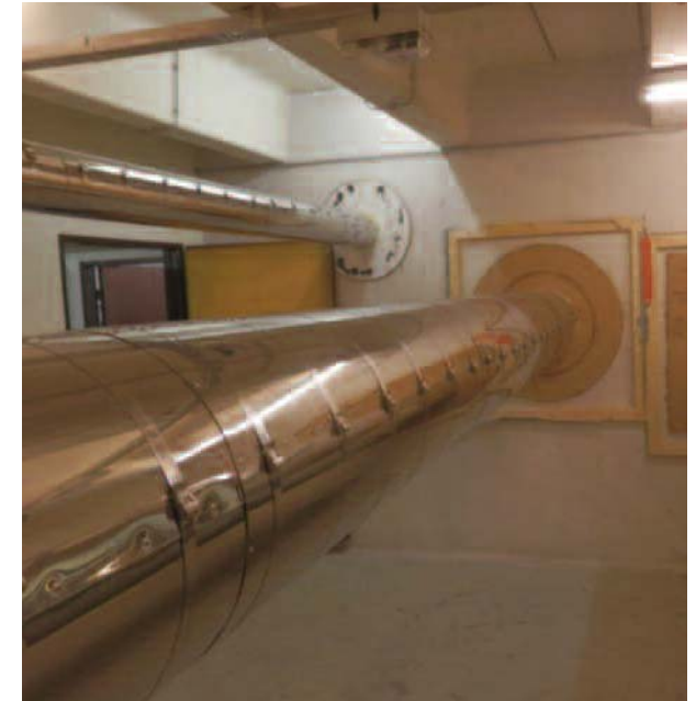
Typical test arrangement of pipes tested insulated with the FireMaster pipe fire protection system
